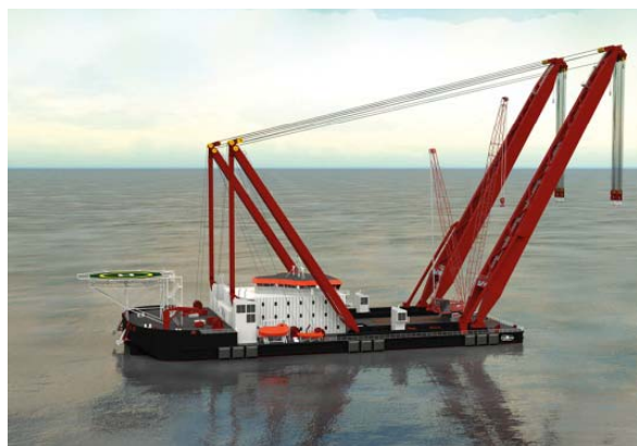
Gulliver Self-propelled crane ship (4,000 T)
