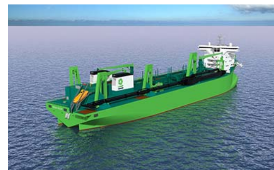
Bonny River - Trailing suction hopper dredger (14,500 m 3 )
